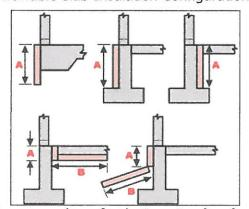
A or A+B must equal two feet in Zone 5 or four feet in Zone 6
